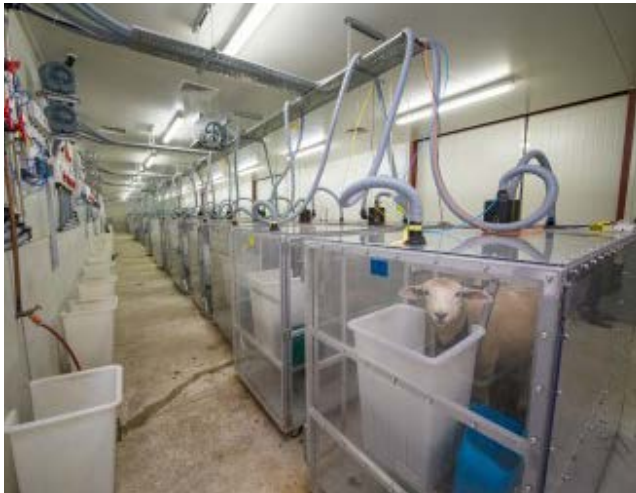
Sheep having their methane measured in respiration chambers https://www.nzagrc.org.nz/domestic/methane-research-programme/the-science-of-methane/
