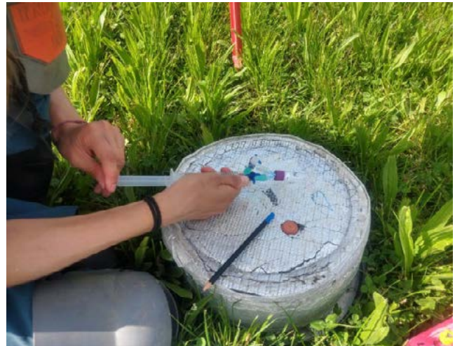
Measuring nitrous oxide emissions in the field https://www.nzagrc.org.nz/domestic/nitrous-oxide-research-programme/plants-and-nitrous-oxide-emissions/
